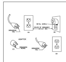
WARNING: This heater has a voltage rating of 120 volts. The cord has a plug as shown in A. An adapter as shown in C is available for connecting three-blade grounding-type plugs to two-slot receptacles. The grounding lug extending from the adapter must be connected to a permanent ground such as a properly grounded outlet box. The adapter should not be used if a three-slot grounded receptacle is available.
