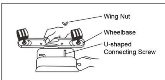
1. Remove the heater body, two wheelbases, and two U-shaped connecting screws with wing nuts from the box. Remove the packaging materials and keep for future storage.
